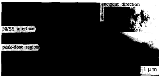
Fig. 1. A typical micrograph of a cross-sectional foils from the solution-annealed specimen implanted at 550°C.
